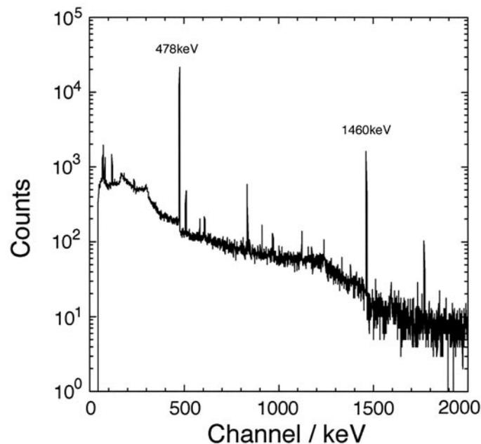
Fig.3. Typical  $\gamma$ -ray spectrum of the  ${}^7\text{Be}$  in the sample of Be metal.
