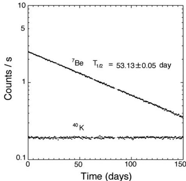
Fig.4. Exponential decay line of  ${}^7\text{Be}$  in the sample of Be metal ( ${}^7\text{Be}$ ). Background radioactivities of  ${}^{40}\text{K}$  are also shown in the figure.
